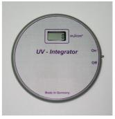
By addition of the incidence of the light quantities during the exposure cycle, relative values are calculated.
