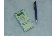
The UV-MICROLOG D is a small, only 6 mm flat, self-contained, pass-trough UV data logging unit. It is specially designed to measure, record and display peak UV intensity, UV dosage and temperature in the UV curing process of narrow web presses and in some applications of the flexo print. It is equipped with one UV sensor and one temperature sensor for the individual measuring of
