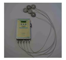
The Data Sampler PL2516 SD is a small, portable, pass-through, UV & temperature data sampling unit for UV & IR Curing systems, UV & IR Profile Analysing and 3D-UV & IR Data Acquisition. It has been specifically designed to measure UV-radiation and temperature on high-end UV-IR curing machines.
