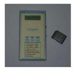
The **UV-4C Microlog 10 with SD Memory card** is a self-contained, high quality UV measuring instrument. It is designed to measure, record and display peak UV intensity, UV dosage and temperature in the UV curing process.
