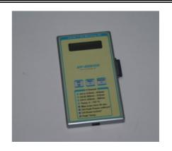
The **UV-T Microlog 10 with SD Memory card** is a self-contained, high quality UV measuring instrument. It is designed to measure, record and display peak UV intensity, UV dosage and temperature in the UV curing process.
