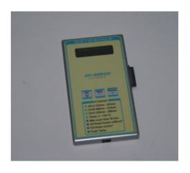
The *UV-3C Microlog 10 with SD Memory card* is a self-contained, high quality UV measuring instrument. It is designed to measure, record and display peak UV intensity, UV dosage and temperature in the UV curing process.
