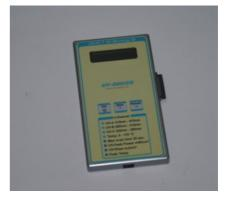
The **UV Microlog 10 with SD Memory card** is a self-contained, high quality UV measuring instrument. It is designed to measure, record and display peak UV intensity, UV dosage and temperature in the UV curing process.
