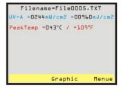
Due to its UV sensors and the integrated microprocessor the **UV-1060 Colour RE Radiometer + Dosimeter RE** can measure, record and display the peak of the UV-intensity (mW/cm<sup>2</sup>) plus the peak of total UV energy.
