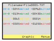
With these four different UV-bands most of the measuring requirements of UV curing applications can be covered.
