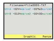
With these two different UV-bands many of the measuring requirements of UV curing applications can be covered. Due to its two different UV sensors and the integrated microprocessor the *UV-1210 Colour RE Radiometer* + *Dosimeter* can measure, record and display the peak of the UV-intensity (mW/cm²) for each UV-band individually plus the peak of total UV energy.
