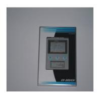
The **UV-1210 Colour RE Radiometer + Dosimeter** is a self-contained, high quality UV measuring instrument. It is designed to measure and record UV intensity, UV dosage and temperature in the UV curing process. Measuring results are indicated both, graphically and numerically on a big colour display.
