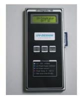
The UV Integrator 160 is a small, self-contained, high quality UV measuring instrument. It is designed to measure and display peak UV intensity in mW/cm<sup>2</sup>, UV dosage in mJ/cm<sup>2</sup> and temperature in the UV curing process.
