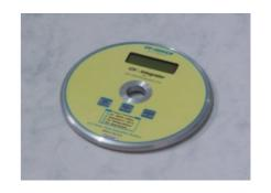
The UV-T Integrator DVD is a self-contained, high quality UV measuring instrument. It is specially designed to measure, record and display peak UV intensity, UV dosage and temperature in the UV curing process of CD and DVD production.
