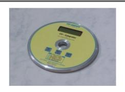
The UV-Integrator DVD is a self-contained, high quality UV measuring instrument. It is specially designed to measure, record and display peak UV intensity and UV dosage in the UV curing process of CD and DVD production.
