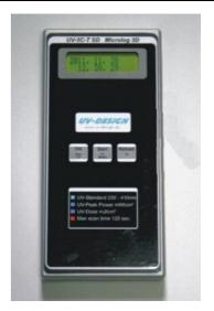
The UV-2C Power Integrator is a small, self-contained, high quality UV measuring instrument. It is designed to measure, record and display peak UV intensity (mW/cm²), UV dosage (mJ/cm²) and temperature in the UV curing process.
