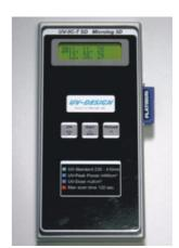
The UV-4C Microlog SD with SD Memory card is a self-contained, high quality UV measuring instrument. It is designed to measure, record and display peak UV intensity, UV dosage and temperature in the UV curing process. It is equipped withfour different UV sensors and one temperature sensor for the individual measuring of
