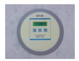
The UV-3C Microprocessor Integrator is a self-contained, high quality UV measuring instrument. It is designed to measure, record and display peak UV intensity and UV dosage in the UV curing process.
